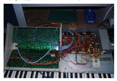
In this picture you can see the rerouted CPU Board connections. coloured running cables from bottom centre of rightboard hand to the Expansion connector and the new trigger cable, blue ribbon cable running from the left-hand board to the Expansion connector.
