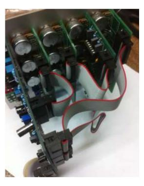
Complete final assembly of the module by mounting all 5 assemblies to the front panel and connect using the supplied IDC cables.
